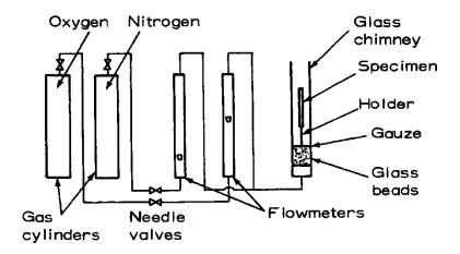
FIG. 1 A - GENERAL ARRANGEMENT OF FLAMMABILITY TEST APPARATUS
