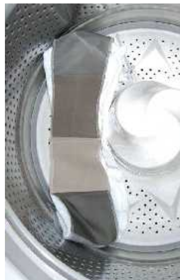
Figure H.11 – Vertical axis washing machine: placement of items in the drum
