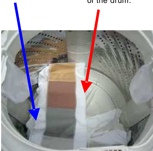
Figure H.11 – Vertical axis washing machine: placement of items in the drum
