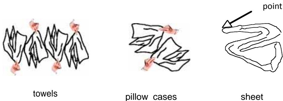
Figure H.12 – Horizontal axis washing machine: illustration of alternating orientation
