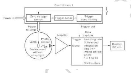
FIGURE C1 - TYPICAL SET-UP FOR RUN-UP TIME TEST
