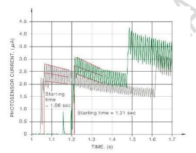
FIGURE B2 - DIAGRAM FOR STARTING TIME (EXAMPLES 1& 2)
