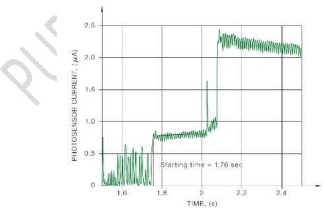
FIGURE B3 – DIAGRAM FOR STARTING TIME (EXAMPLE 3)
